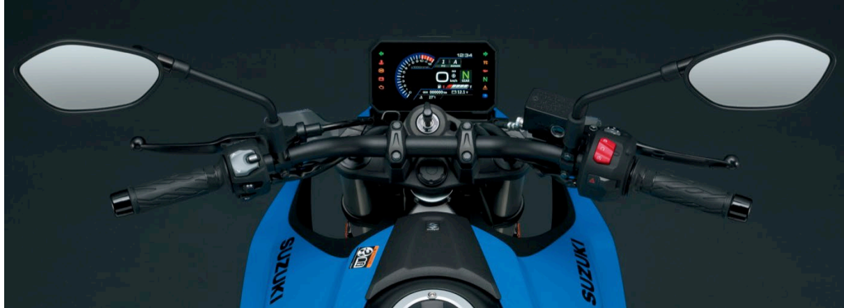
Tapered Aluminum Handlebars
