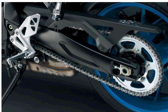
Uniquely Shaped Lightweight Aluminum Swingarm
